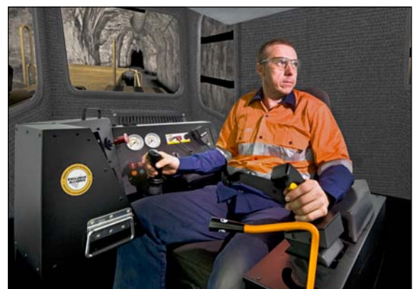
Advanced Equipment Simulator UG360
